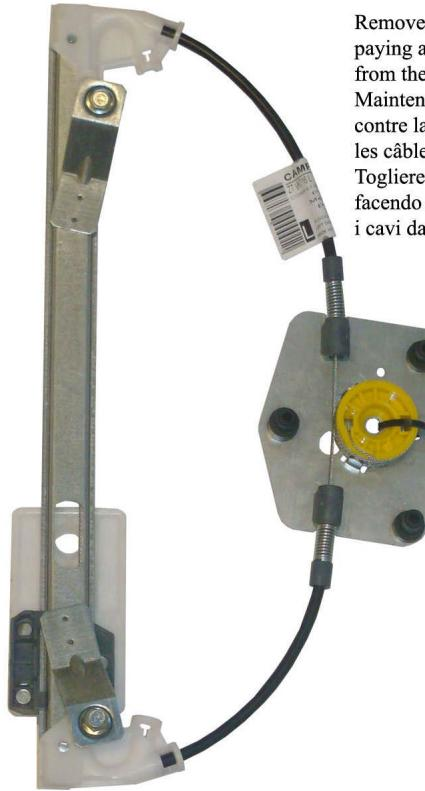
Remove the gear pvc clamp,
